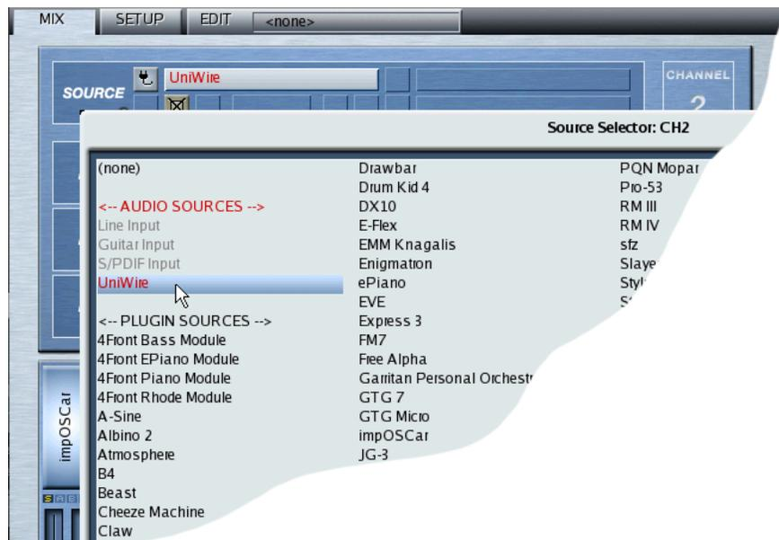
*The previous illustration shows how to accomplish this with Receptor's graphical interface. To do this on Receptor's front panel, set Receptor to the desired channel (see your Receptor manual), press the SOURCE button, rotate the top display knob to select the SOURCE parameter and rotate the bottom display knob to select UniWire. Press the bottom display knob to apply your selection.*
