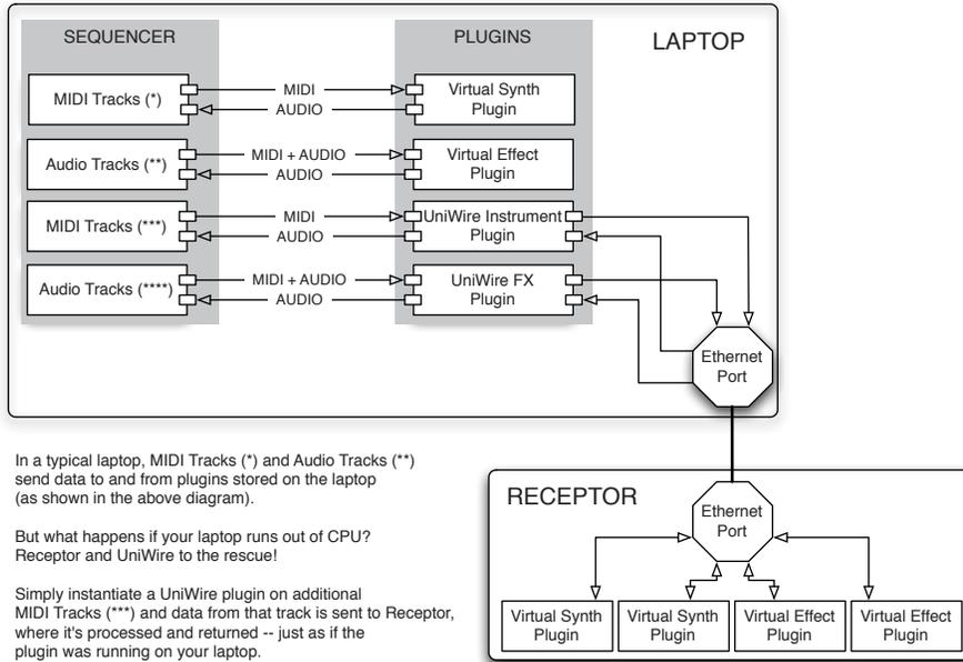
In a typical laptop, MIDI Tracks (\*) and Audio Tracks (\*\*) send data to and from plugins stored on the laptop (as shown in the above diagram).
