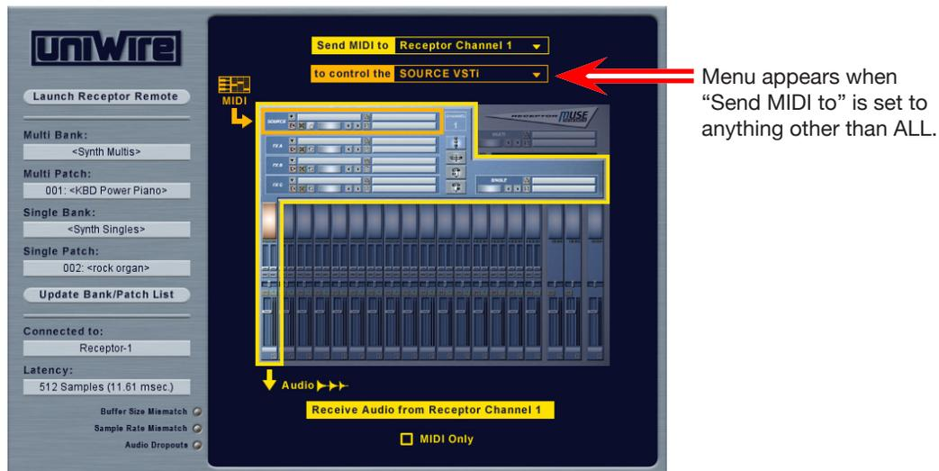
Note that the name of this menu varies slightly depending on whether you're using a UniWire Instrument or an FX. If you're using an instrument, the parameter is called "To control the." If you're using an FX, the parameter is called "MIDI Controls." The functions, however, are nearly identical.
