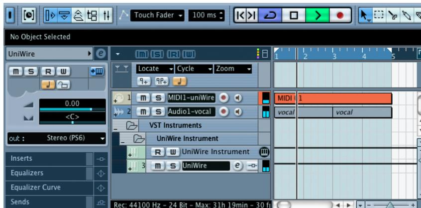
Notice that, in this example, both tracks are bussed to the same audio outputs (“Stereo (PS6)” in this case)
