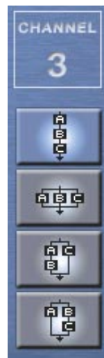
The three insert effects can be arranged as any one of four different configurations.
